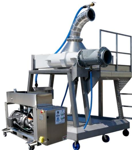
Indoor RAS setup with elevated BP120 skid, auto priming and mobile hydraulic power unit, transferring 4-6kg Atlantic Salmon from growout to purge.
